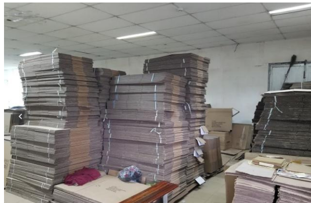
Figure 9: Excessive Storage of Combustible Packaging
