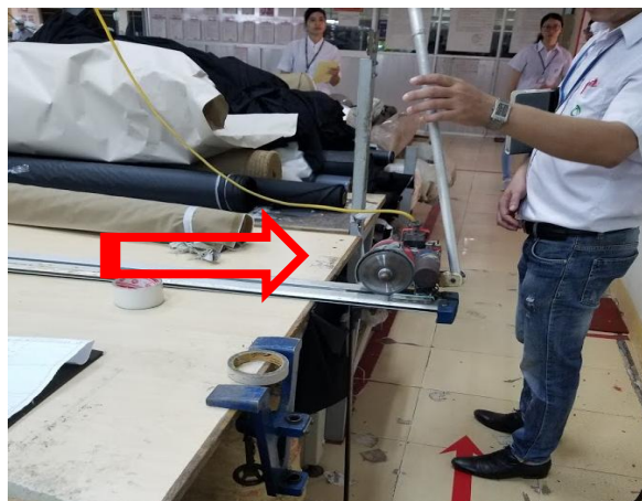
Figure 15: Unguarded Cutting Blade
