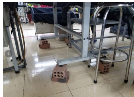
Figure 26: Worktable Propped Up on Bricks
