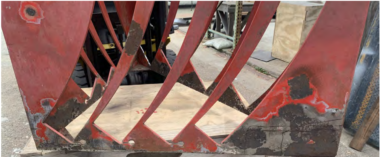
Detail of Short Side Without Signature After Grinding. Areas to be Replaced are Marked
