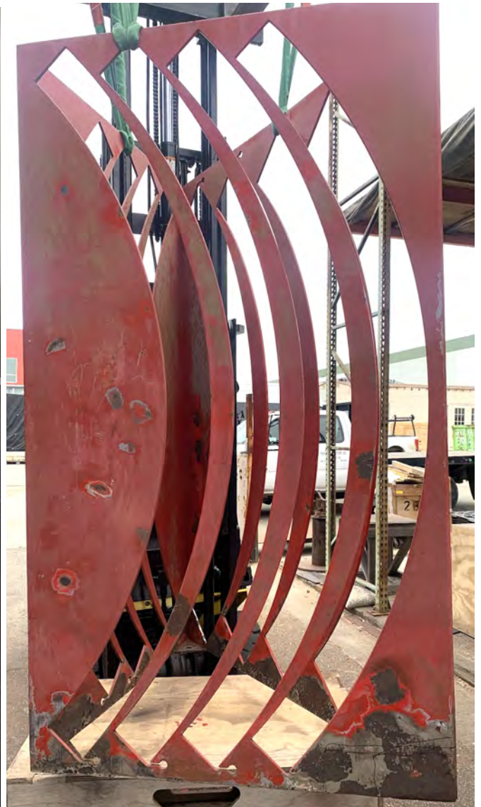
Long Side (Left) and Short Side Without Signature (Right) After Grinding. Areas to be removed are marked with Sharpie Pen
