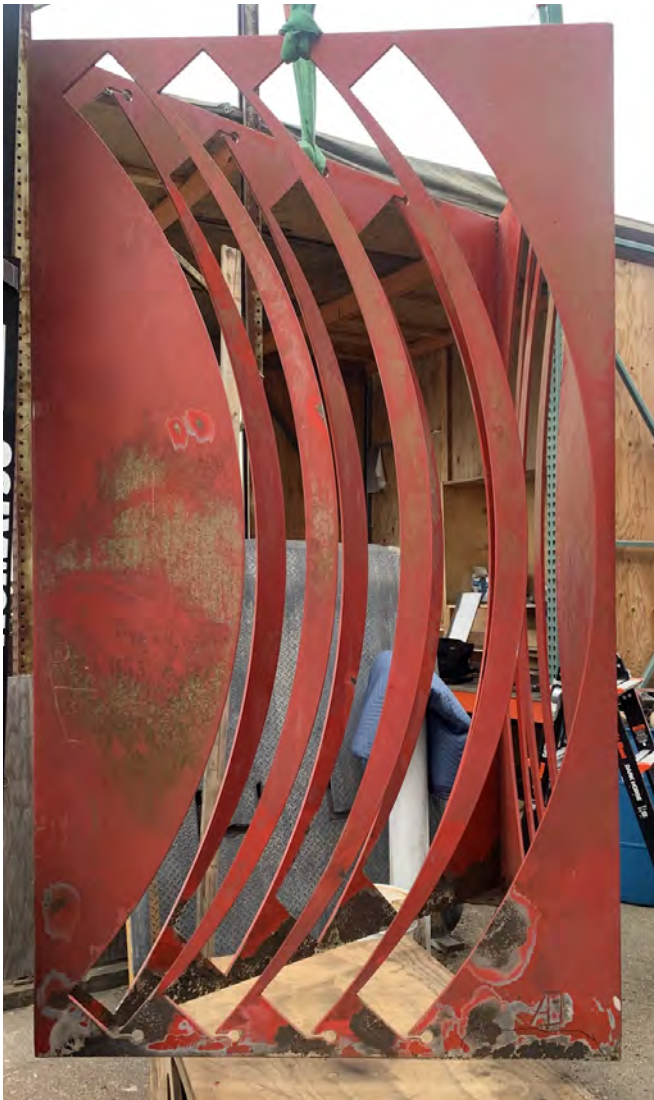
Signature Side After Grinding. Areas Marked with Sharpie Were Replaced (Left) Detail of Corner with Ground Metal (Right)
