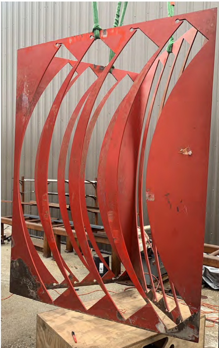
Long Side (Left) and Short Side Without Signature (Right) After Grinding. Areas to be removed are marked with Sharpie Pen
