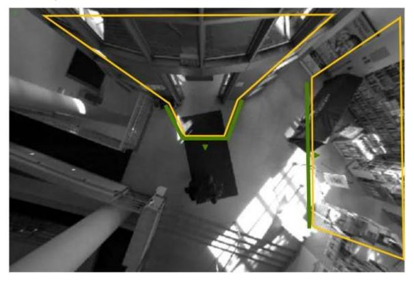
The sensors know their mounted height from the floor and that its individual lenses are 3" apart. It then uses trigonometry to create a Stereo Height map from the 2 images it sees. It then monitors the resulting Stereo height map for anomalies, as in the case of something moving through the scene:
