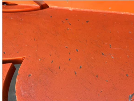
Image 5: Detail view of the orange bench showing repeated impact damage with chips, scratching, and corrosion present.
