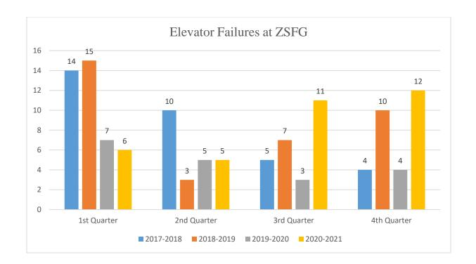
**AIM:** For FY 2021-22 continue to manage and monitor outage trends with an overall goal to manage overall elevator outages. Note: the most common cause of elevator outage was damaged doors to the Bldg 5 cargo elevators (19 & 20). These elevator car doors are often hit by material moved in and out of the elevator (11 of 34 outages).
