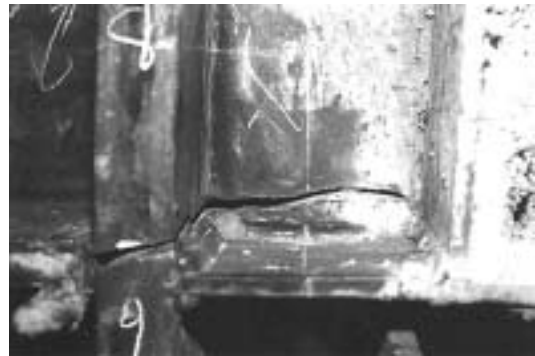
b. Fracture Progresses into Column Web
