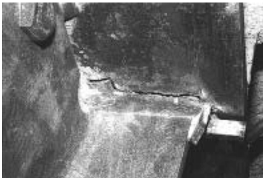
a. Fracture at Fused Zone
