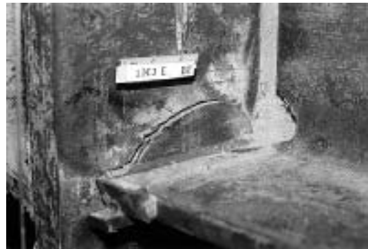
b. Column Flange "Divot" Fracture
