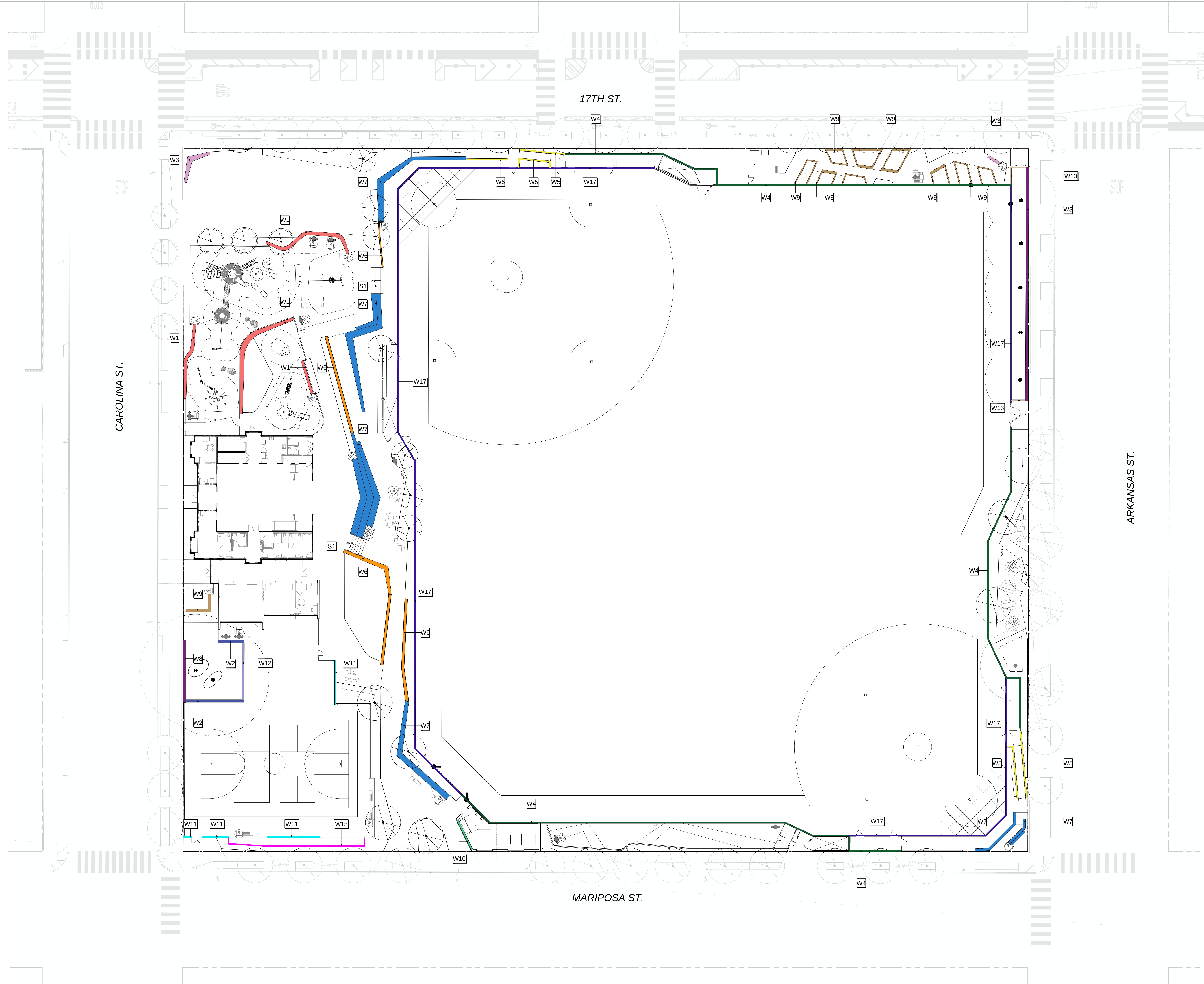
1 ONSITE WALL MATERIALS PLAN
