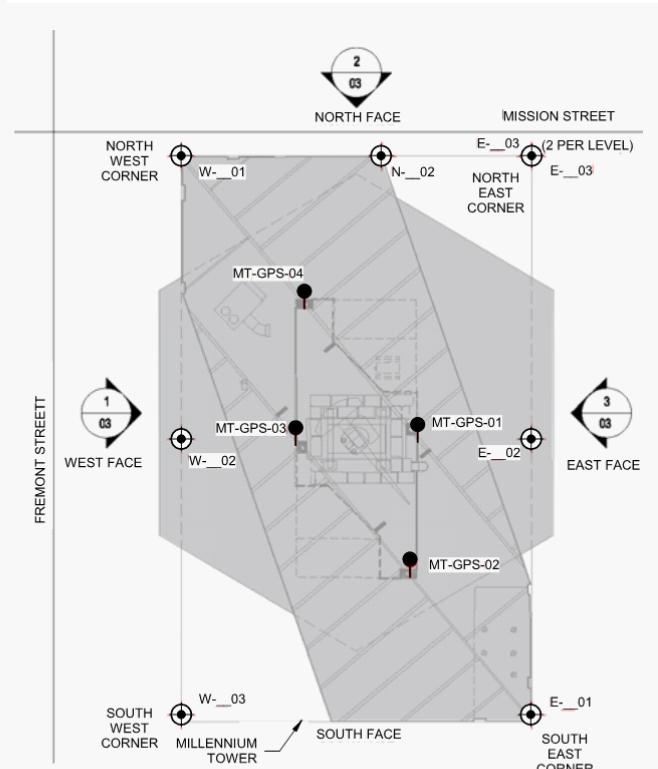
**3 ROOF PLAN OF SURVEY PRISM INSTRUMENTATION** NTS
