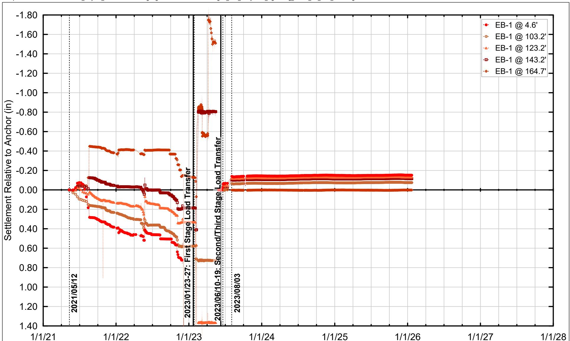
Note: EB-1 was repaired and reset on 2023/05/30
