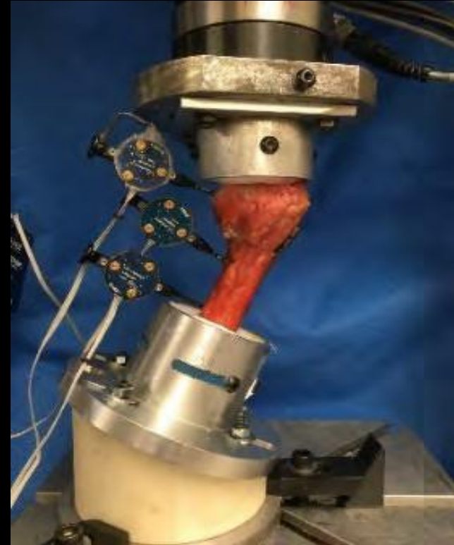
Mechanical comparison of augmentation techniques for locking plate fixation of proximal humerus fractures
