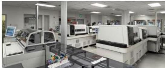
paired with go-live for the automated track for Chemistry and Hematology instruments. This automated track utilizes amazing robotics and software that guide specimen tubes around the track so they can be centrifuged, uncapped, sampled at each instrument, tested on the instruments, and then recapped and stored in a refrigeration unit. Meanwhile test results flow from instruments into Beaker and then into Epic where providers can see results.
